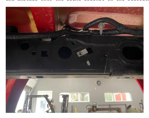
Shown bellow is the nut/clip installed on the relocation kit.
