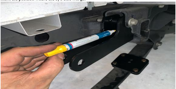
Drill a 3/8 hole thru the chassis. See picture for reference.
