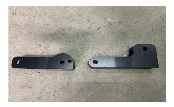
Pictured above on the Right is the drivers bracket and on the left is the passenger side bracket. These brackets require a single 3/8 hole to be drilled to keep the mounts secured to the chassis.
