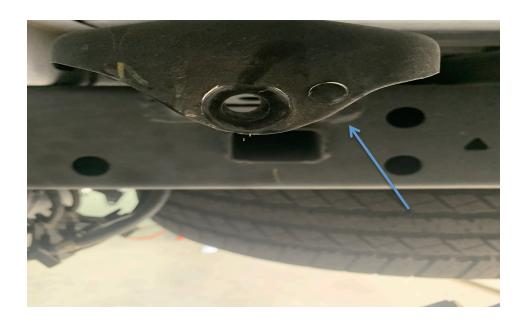
Next install the Passenger side relocation mount. Insert the mount into the factory shock location with OEM shock bolt. Do not tighten down yet. With the mount-installed loosely, mark the position where the 3/8 bolt will go.
