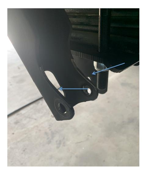
Drill out the lower shock mounts to  $\frac{1}{2}$  hole and install the Viking shocks using the  $\frac{1}{2}$  sleeves provided by Viking. The Viking shocks are 1.25" wide and will require 3 washers (provided with the kit) between the shock and inner shock mount to fill in the gap. Use the provided bolts and washers and torque to 60ftlbs. This is true for both passenger and driver lower mounts only.
