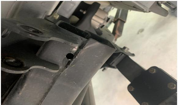
Next install the passenger side mount with the factory shock bolt. Use a long extention and instert the provided 3/8 bolt and nylon lock nut and torque to 35 ftlbs.
